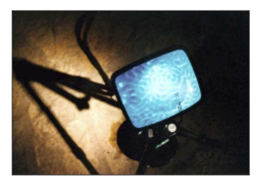
...a loudspeaker filled with water is connected to an audio signal, so that changing structures can be seen on the water's surface. This is recorded onto a miniature camera and returned to a cathode-raytube. Light emissions from the tube are transformed into an electronic signal using a light-voltagetransformer. This signal is then sent to theloudspeaker via an audio amplifier...
